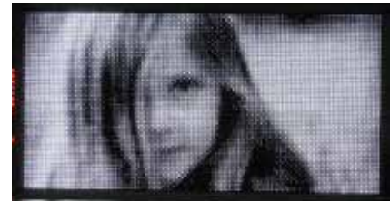
White LED Module + Cabinet pixels: 64h x 128w dimension: 32"h x 64"w
